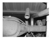
INSTALL DRIVERS SIDE FRONT TAILPIPE # D INTO MUFFLER 1-1/2" TO 2". USE CLAMP # I AND ATTACH IT TO THE MUFFLER. DO NOT TIGHTEN.
