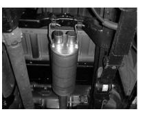
INSTALL MUFFLER #B ONTO HEADPIPE 1-1/2" TO 2" USING CLAMP #J. INSERT WELDED HANGERS INTO RUBBER GROMMET. MAKE SURE OUTLETS ARE LEVEL. USE A JACKSTAND TO SUPPORT MUFFLER.
