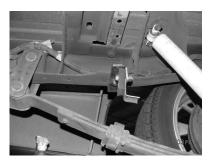
INSTALL HANGER # F ON THE PASSENGER TAILPIPE AND HANGER # G ON DRIVERSIDE TAILPIPE. MEASURE 19" FROM REAR OF FRAME AND BOLT INTO THE EXISTING ROUND HOLES (ABOUT 7/8") LOCATED ON THE FRAME ON BOTH SIDES
