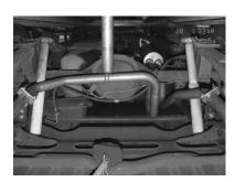
INSTALL DRIVERS SIDE OVERAXLE PIPE # E ONTO FRONT TAILPIPE USING CLAMP #I. USE CLAMP # I TO HOLD TAILPIPE UP TO REAR HANGER # G. DO NOT TIGHTEN.
